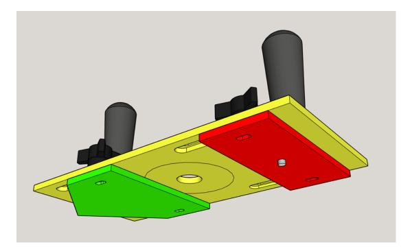
To cut a circle WITHOUT drilling a hole into the center of your workpiece, leave the set up the same as above, and add another Extension Foot (C) onto the Triangle Base (B) (pictured below on the left.)
