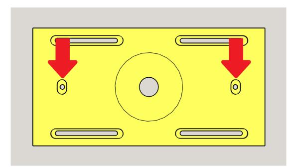
It is easy to do this step with the baseplate on a flat surface. The head of the T-Bolts will lock into place in the recessed holes on the underside of the Base Plate when twisting on the handles.
