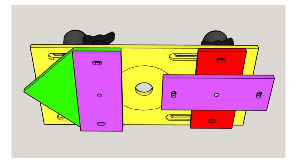
(Note: If you are cutting a smaller diameter circle, like 3", that double stick taped extension foot might be too big, just cut a scrap of 1/4" thick material that is smaller and drill and 1/4" hole into it. Then you can double stick tape that to your workpiece and use it as your pivot point.)
