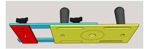
OR you can make larger circles WITHOUT drilling a hole in the center by adding the Triangle Base (B) to one side of the Main Base (A), double stick tape one of the Extension Feet (C) to your workpiece and rotating around that!
